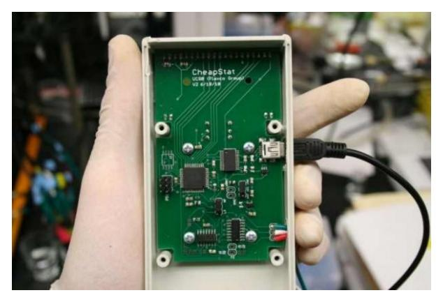
A potentiostat is an electronic instrument that controls the voltage difference between a Working Electrode and a Reference Electrode contained in an electrochemical cell. Control is achieved by injecting current into the cell through an Auxiliary, or Counter, electrode.
