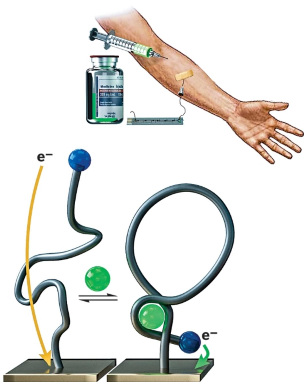
MEDIC chip (top) would be connected to patient's bloodstream to continuously measure a target drug. Inside the device (illustrated at bottom), binding of target (green sphere) to aptamer (gray) causes shape change that boosts electron-transfer rate (curvy arrows) from an electrochemical reporter (blue) to gold electrode (rectangular base), generating detection signal.
